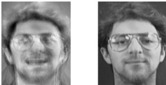
Figure 1: An image recovered using a new model inversion attack (left) and a training set image of the victim (right). The attacker is given only the person's name and access to a facial recognition system that returns a class confidence score.
